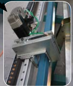
High Accuracy Bar Feeder with Pneumatic Clamp
